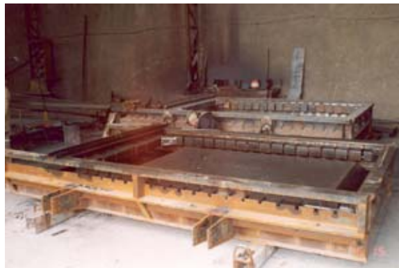
A typical steel mold for concrete pouring – MK Beton mold fabrication facility
