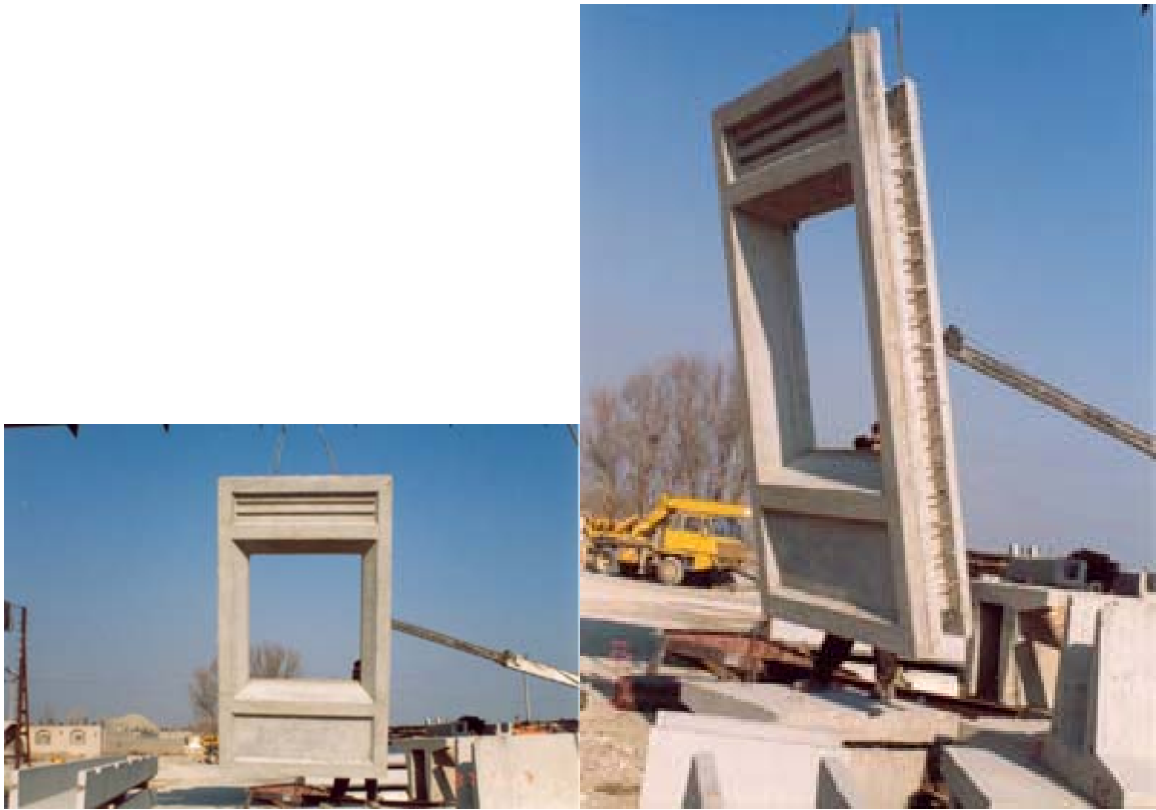
A typical structural window panel – MK Beton's factory site
